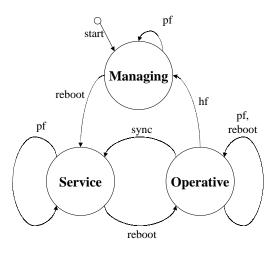
Fig. 2. The FSM describing the OS organization of the MULTISOFT machine
